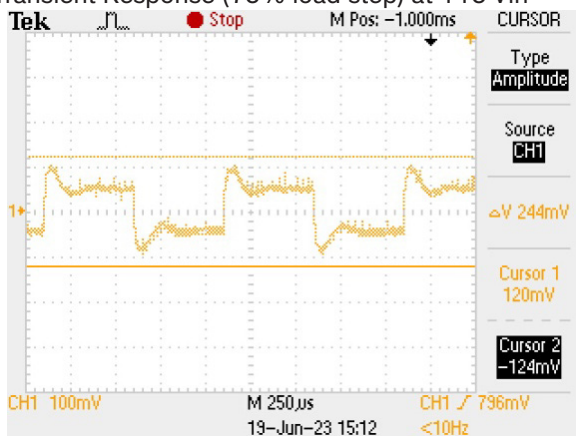
Transient Response (75% load step) at 115 Vin
