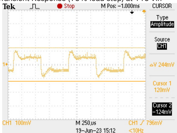
Transient Response (75% load step) at 115 Vin
