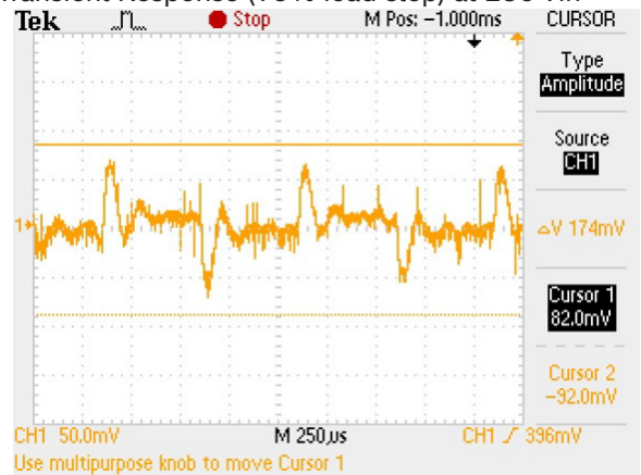
Transient Response (75% load step) at 230 Vin
