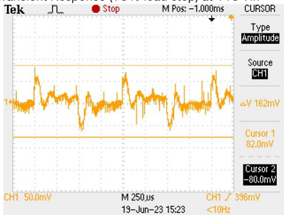
Transient Response (75% load step) at 115 Vin
