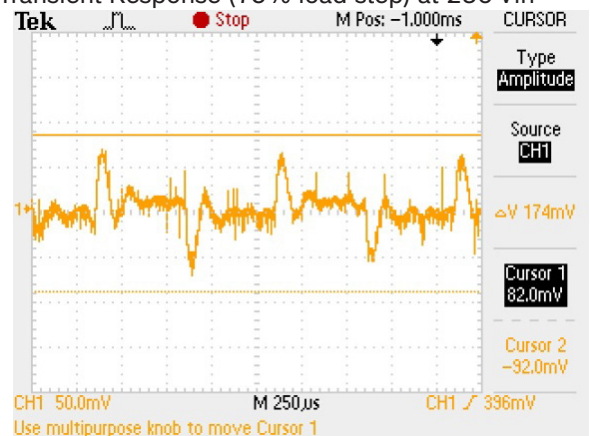
Transient Response (75% load step) at 230 Vin
