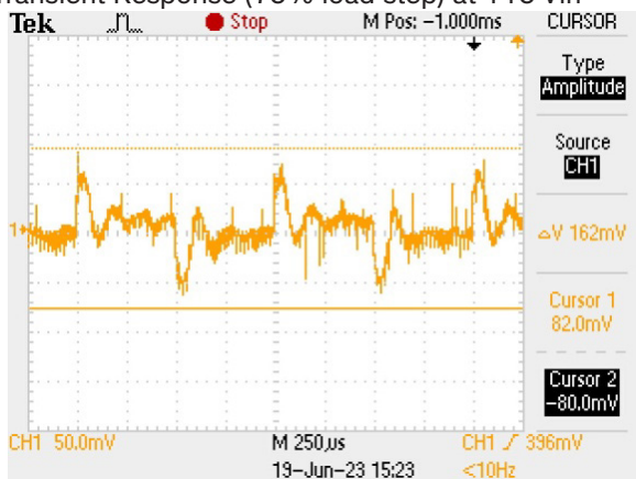
Transient Response (75% load step) at 115 Vin
