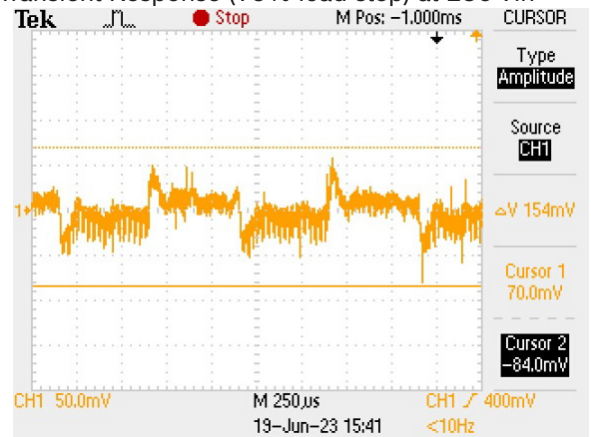
Transient Response (75% load step) at 230 Vin
