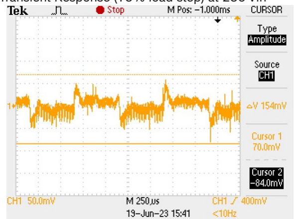
Transient Response (75% load step) at 230 Vin
