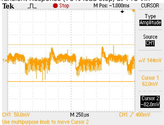
Transient Response (75% load step) at 115 Vin
