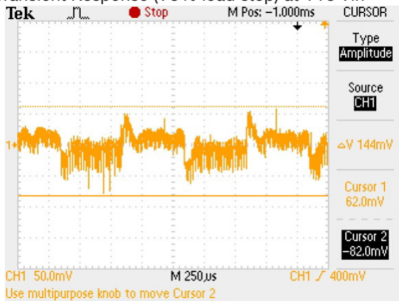
Transient Response (75% load step) at 115 Vin
