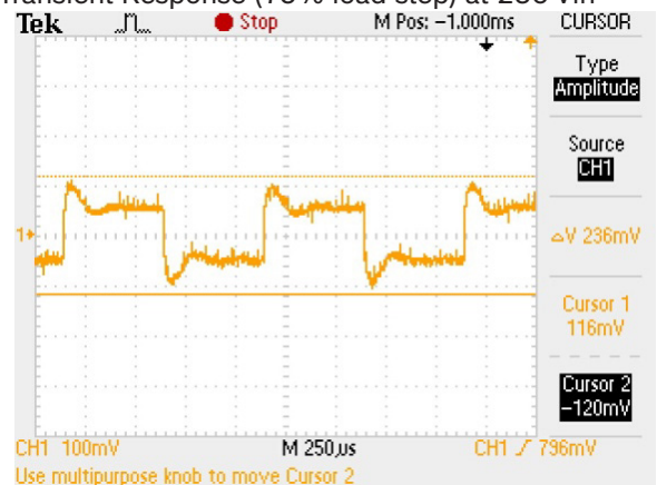
Transient Response (75% load step) at 230 Vin
