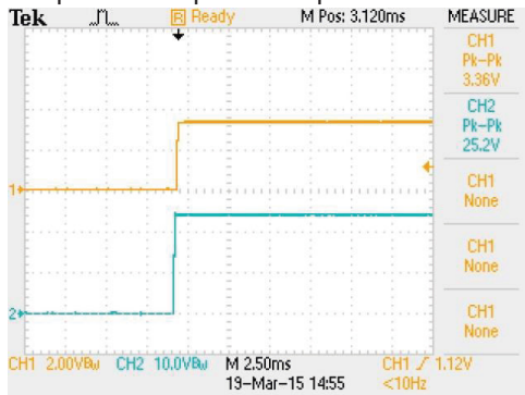
Typical Input Start-Up and Output Rise Characteristic
